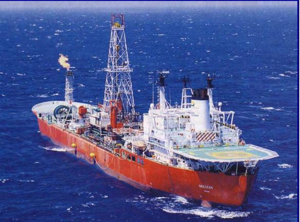
As *Seillean* operated since 1999, this time continuously on station – normal cycle with export tankers being hawser moored or on DP.
