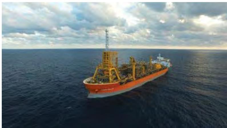
The 900-ft long Turritella is the second FPSO to be moored in the Gulf of Mexico. It is stationed in 9,500 ft of water at Shell's Stone field. Photo from SBM Offshore.
