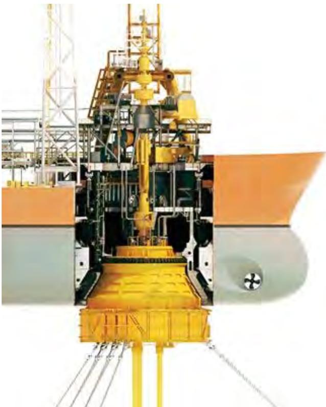
The Turretella features a buoyant turret mooring. The vessel rotates around the turret as wind and currents change. Turretella can disconnect from its buoy, which then drops to a safe depth, if a hurricane approaches. Photo from SBM Offshore.
