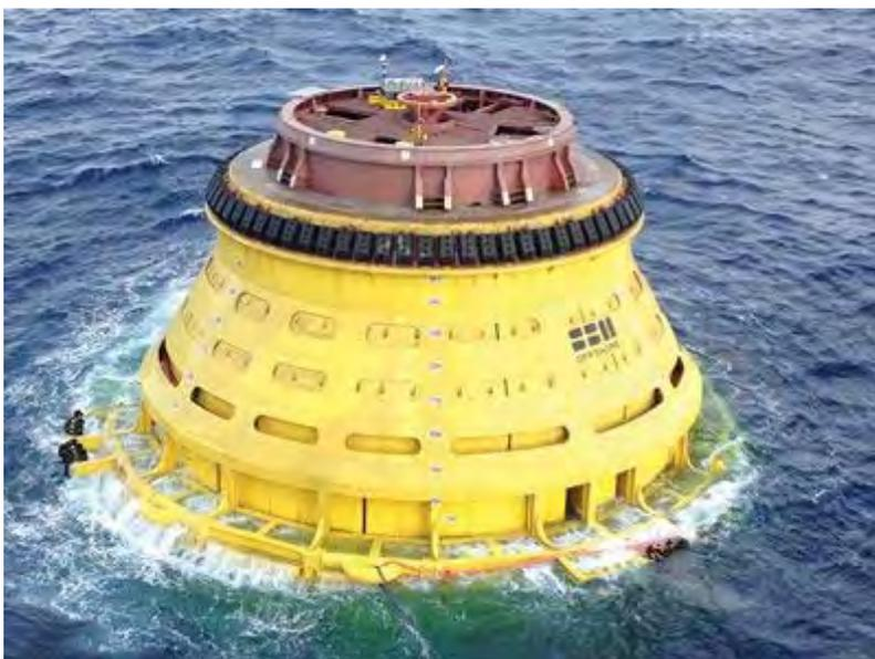
Shell's Stones project features the largest disconnectable buoy built for the oil and gas industry to date. The buoy was designed for use with steel lazy-wave risers. Photo from SBM Offshore.
